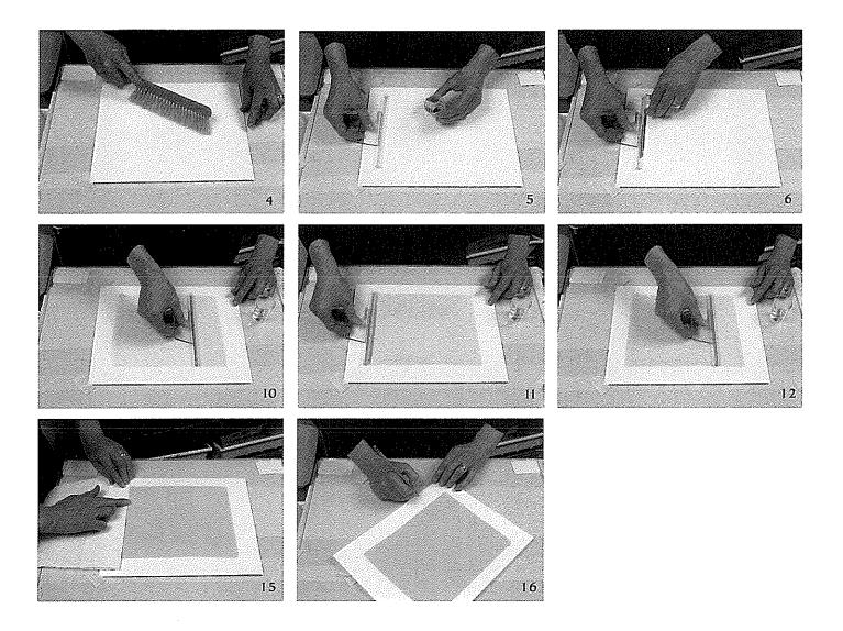
marked area (8). Don't hurry, don't press down, just slide the tube across, stop, and move it back the other way just about one inch. Lift it gently, leaving a puddle (the trade name of one glass tube is "The Puddle Pusher"). Move it back behind the puddle, and then pull it to the starting point again. (9) If you lose the puddle behind the tube, you're moving too fast.
