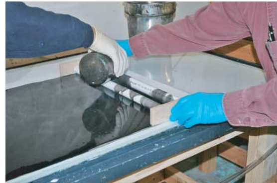
Fig 44. Here is the coating die in use.
