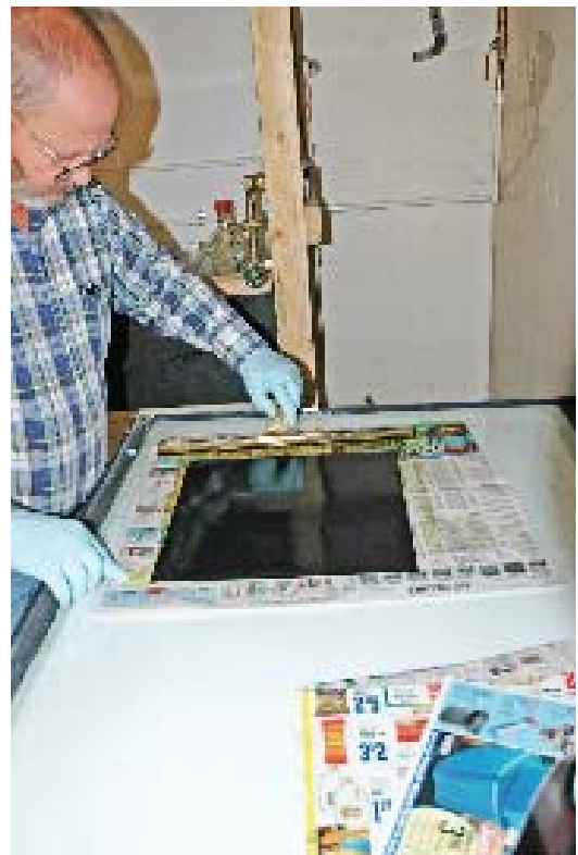
Fig 15. The tissue is now placed on a piece of paper and very gently squeegeed.
